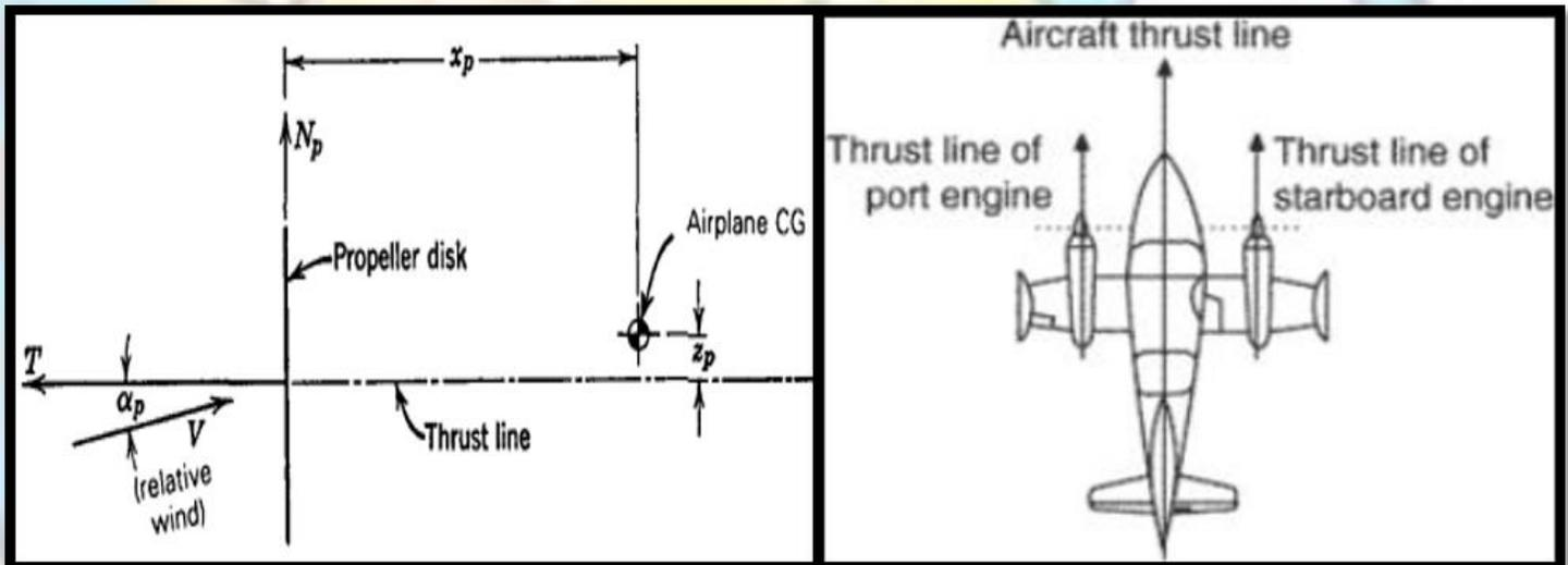
**Longitudinal stability**, by the letter of the law, is defined by whether increasing elevator control force is needed to change and maintain an airspeed, and whether the aircraft returns to the same airspeed with elevator released.
