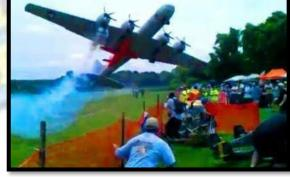
failure (although the photographic image is somewhat blurred the right wing clearly displays the missing aileron) – should a pre-flight check (inspection) have been carried out prior to flight the accident would have been negated.
