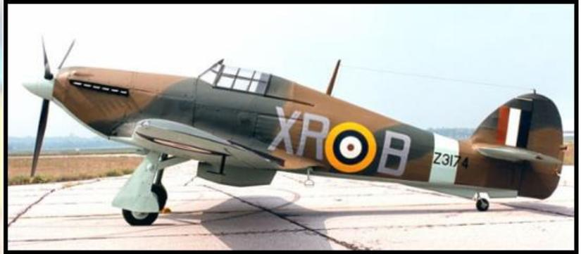
And finally, what's in a design - the **Hawker Hurricane** (top right), evolved from the **Hawker Fury** (left). Designers and Engineers simply took an existing Biplane, the Hawker Fury, removed its upper wing and pimped it out beefing it up where required in preparation for combat service as a single wing fighter. I don't know if that's lazy or innovative – but it is another example of the British work around.
