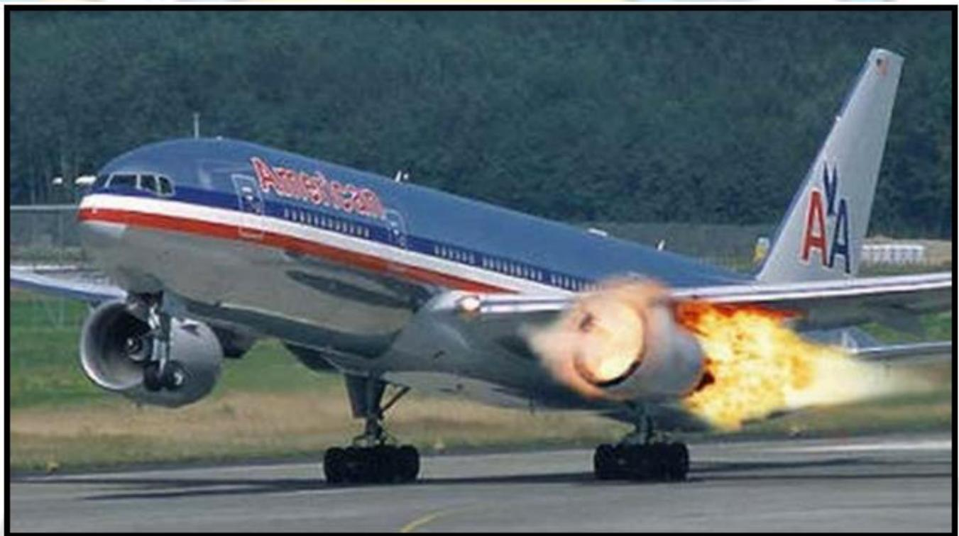
An aircraft does not have to be travelling fast to cause a **Surge** or **Stall** condition.
