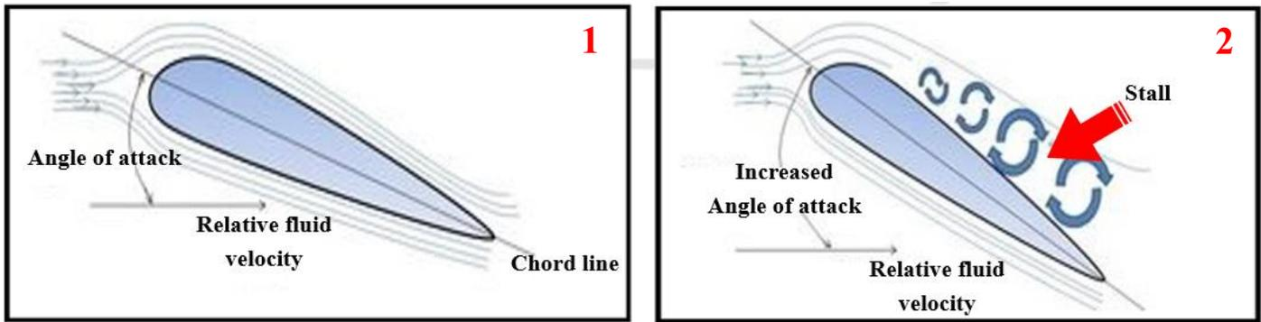
An aerofoil will stall when the airflow completely separates from its top (**Low Pressure**) side.
