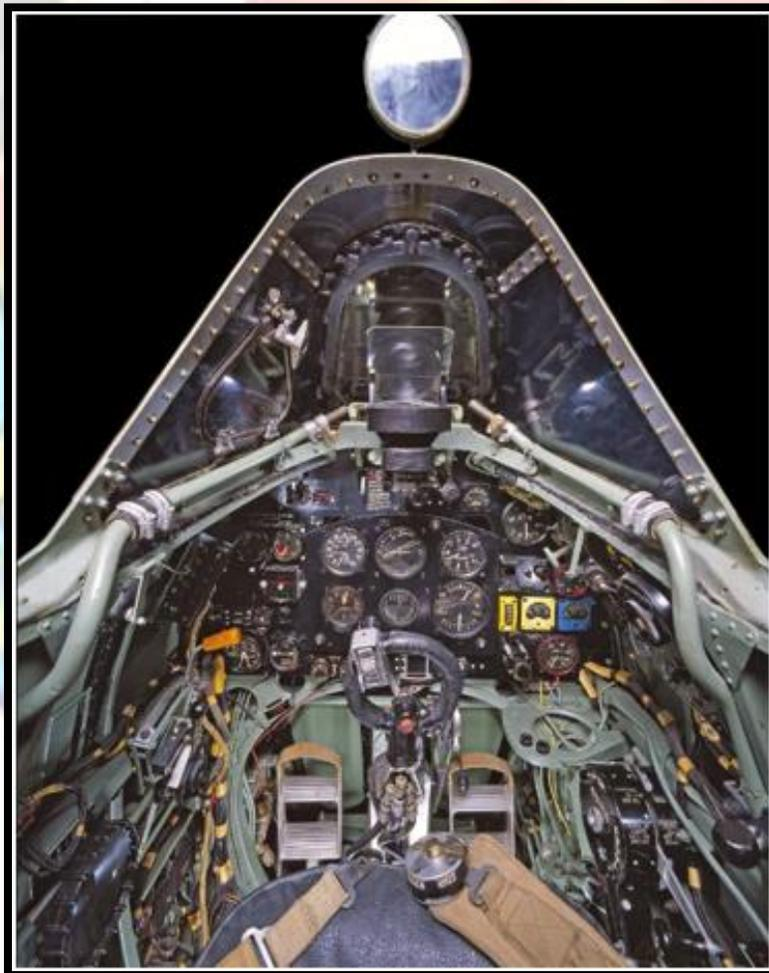
The **Throttle** was fitted similarly adjacent in position on the left or port side of the aircraft in close proximity to a protruding fuselage stiffening rib. Like the manual hand-pump for operating the hydraulic undercarriage both items when operated in haste often led to a condition known as "**Spitfire knuckle**" where pilots skinned their hand on the side of the cockpit.
