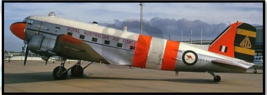
The C-47 **differed** from the civilian DC-3 in **numerous modifications**, which included the fitment of a **cargo door**, **hoist attachment**, and a **strengthened floor**, along with a **shortened tail cone** for **glider-towing shackles**, and an **astrodome** in the cabin roof.
