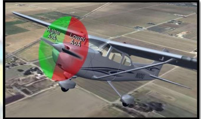
The beauty of the inverted-climb test is that it distinguishes between P-factor and slipstream rotation. To see why, imagine an airplane climbing, and that we are observing from a position behind and above it.
