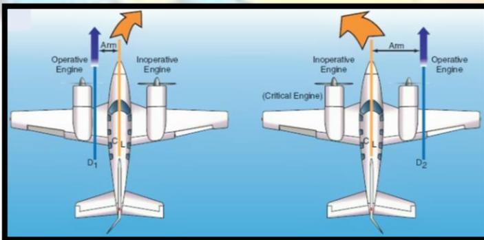
But just sticking to the big first-order effects, consider what happens when the aircraft rolls over and continues its climb inverted. The P-factor force still pulls left because the propeller looks the same when the airplane is upside-down as it did when it was upright. The rudder will still need to be deflected toward our — the observer's — right. But now the pilot (if there was one) is upside-down, and our right would be his left, so he
