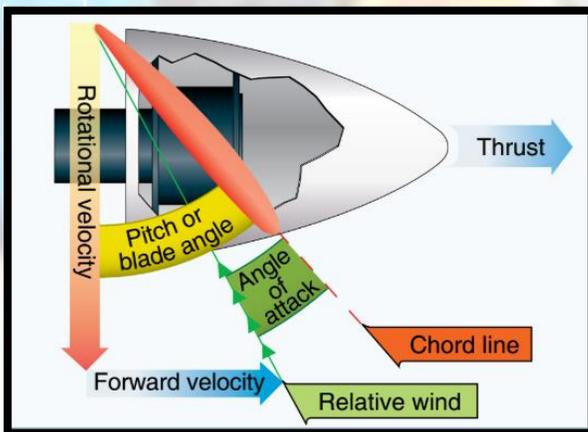
toward the horizontal, the airflow will meet the propeller disc at an increasing angle. The propeller blades moving down and forward (for clockwise rotation, from the one o'clock to the six o'clock position when viewed from the front) will have a **greater** relative wind velocity and therefore will produce greater thrust, while propeller blades moving up and back (from the seven o'clock thru 12 o'clock position) will have a **decreased** relative wind velocity and therefore decreased thrust.
